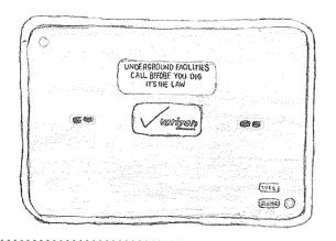
Handholes are structures set belowground that protect telecommunications cables and provide convenient access for splicing or pulling cable. The primary distinction between handholes and other manhole covers is that the former aren't as deep and don't tend to be as crowded as the ducts below manholes.
